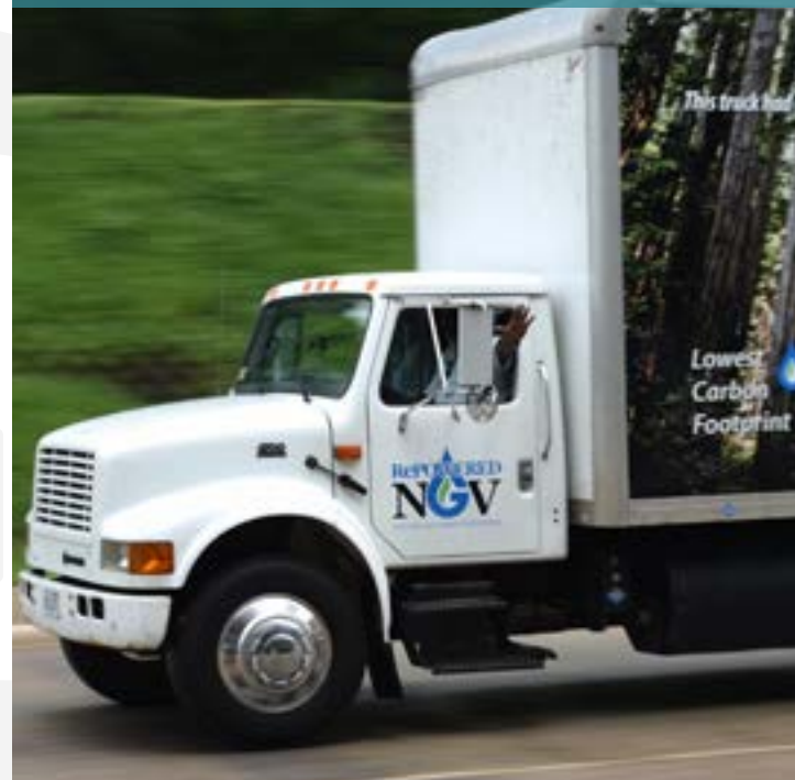
North American Repower unveiled a dedicated-CNG truck with 7.6-liter spark-ignition engine and fuel tanks and assembly by CNG Cylinders International.
