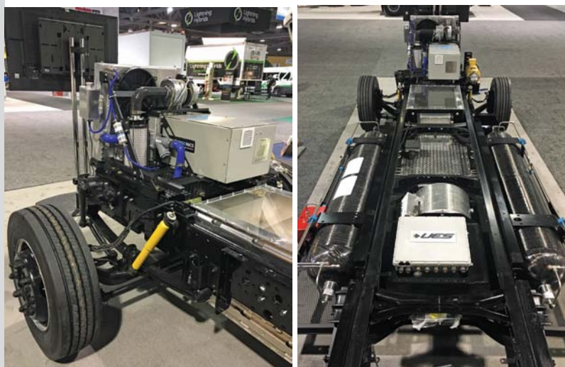
Note Hydrogenics fuel cell and twin fuel cylinders Luxfer ( Booth 837 ) on UPS Class 6 chassis at Booth 1745 .
