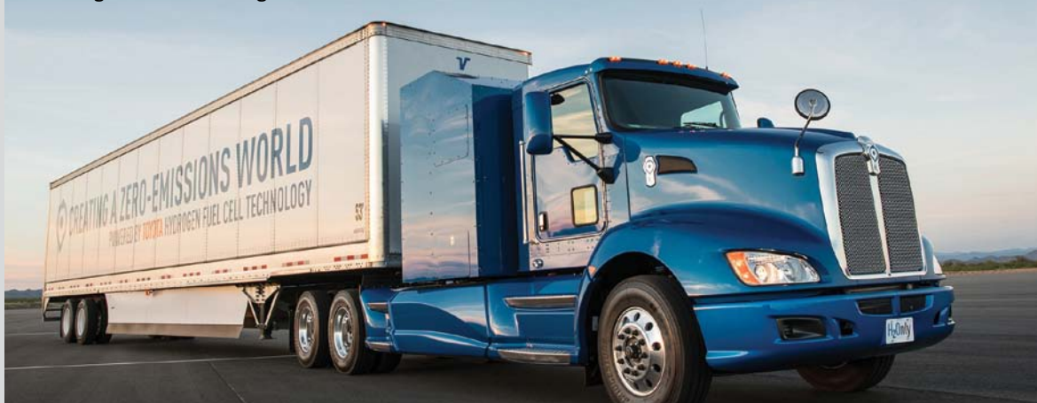
Toyota's 'Project Portal' truck was built using a Kenworth T660 glider.
