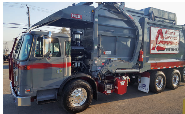
This collection truck for Athens Services is the first Autocar vehicle to be powered by the Cummins Westport ISL G Near Zero engine.
