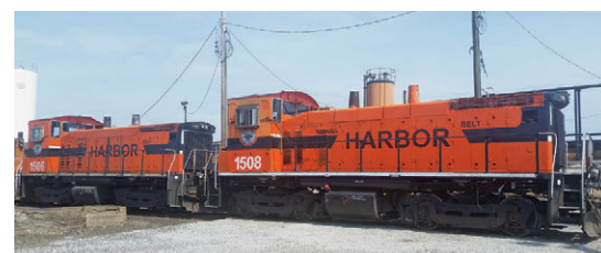
These two Indiana Harbor Belt Railroad locomotives are the first of 21 EMD-built SW1500 units to be converted to CNG-diesel dual fuel operation by OptiFuel and R.J. Corman Railpower. ‘They are currently being built and scheduled to return to IHB in mid-June,’ says IHB mechanical operations director Mike Nicoletti.
