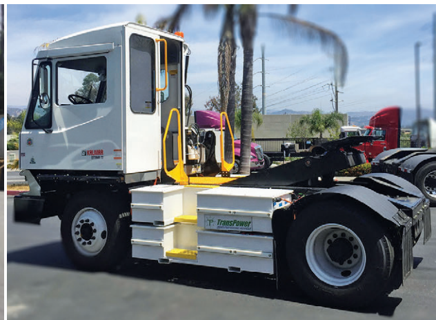
Two views of the 100% battery-electric version of the Kalmar T2 with TransPower drive.
