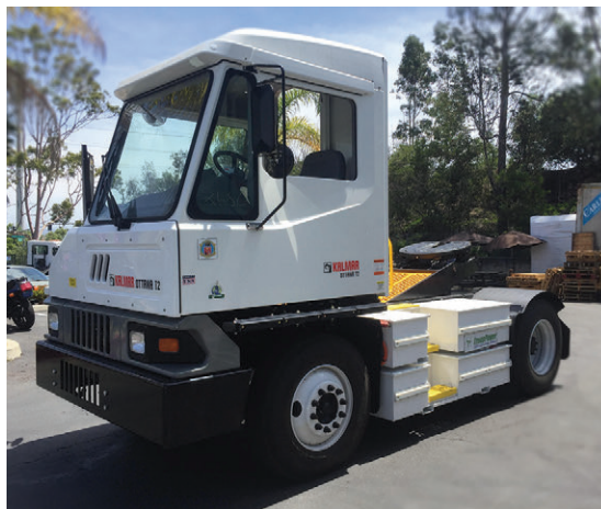
Two views of the 100% battery-electric version of the Kalmar T2 with TransPower drive.
