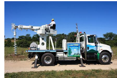
Hybrid Digger Derrick
